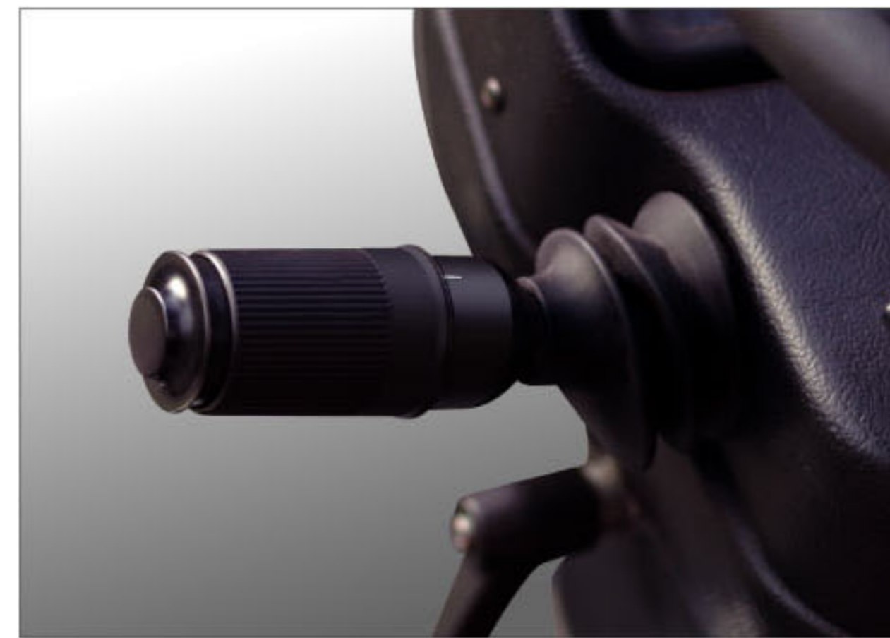
Electric F/R control lever The forward/reverse lever offer easy accessible fingertip control. It is easy to reach and also for fast and easy directional changes. Using the electric solenoid to control F/R is also improved flexibility of operation.
