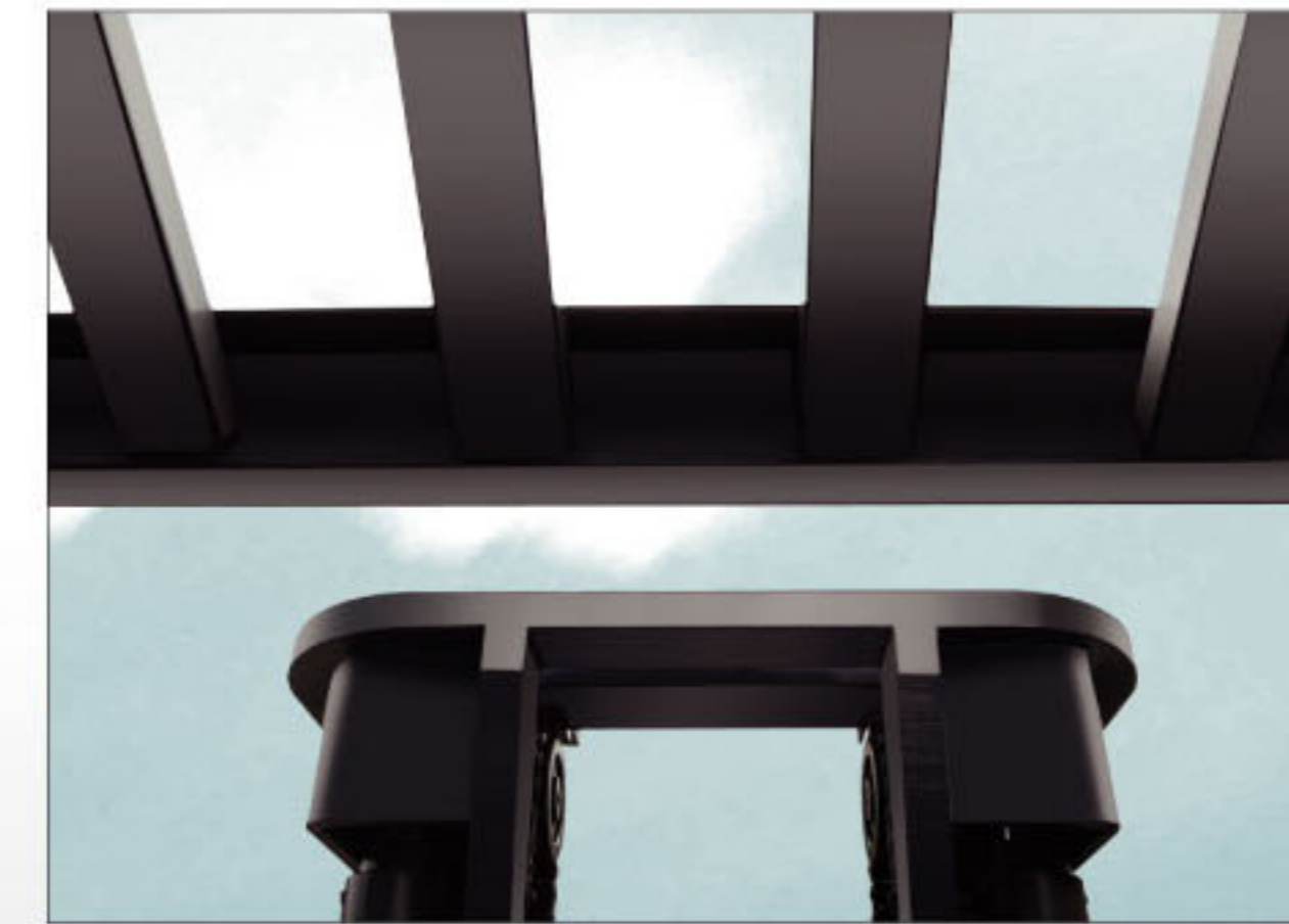
Wide visual head guard Driver gets a best visibility when operates lifting mast upward while watching the mast action.
