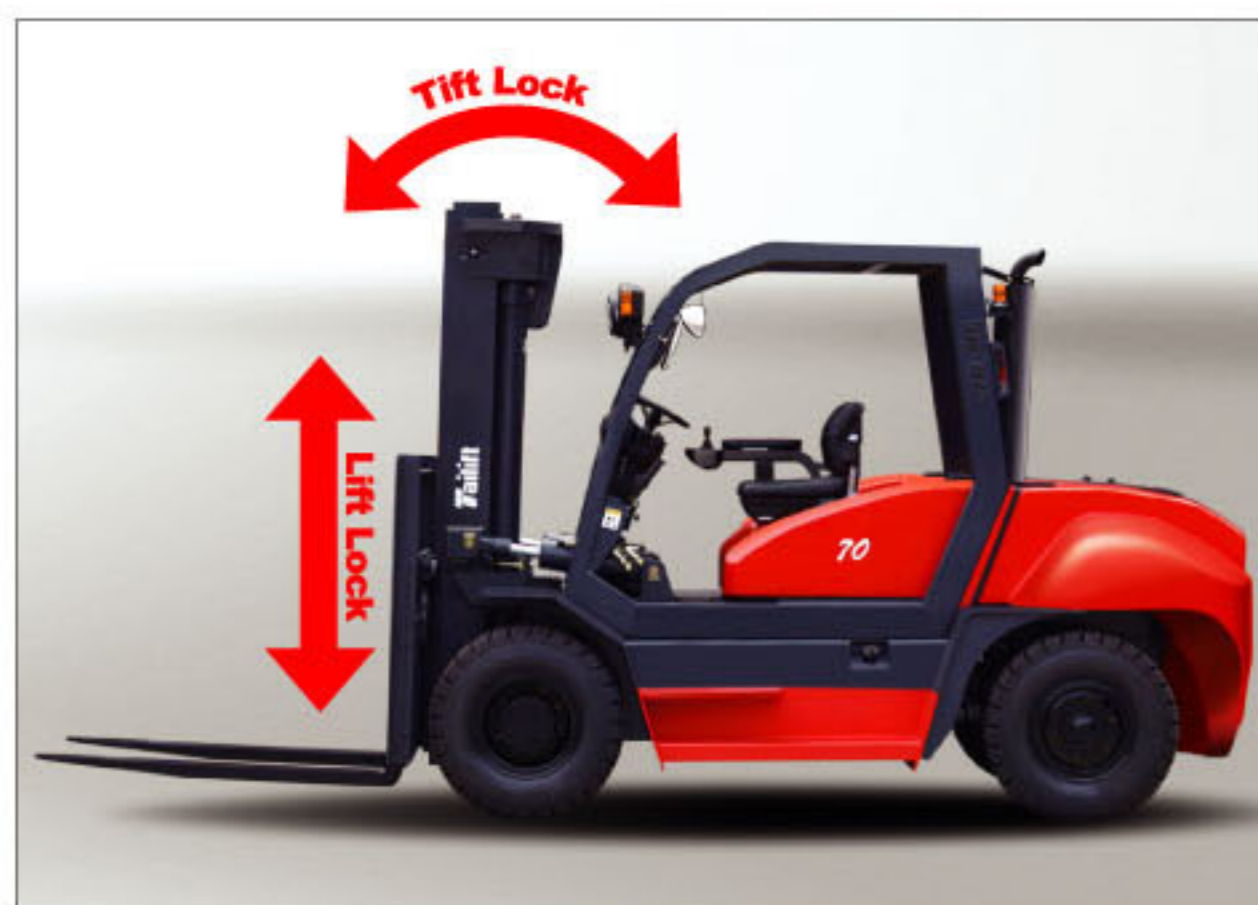
Mast Lock System (optional) The mast lock system automatically locks all lifting and tilting functions when the operator leaves the seat. It is to prevent operator from using the hydraulic functions and driving forklift truck when operator does not seat in proper position.
