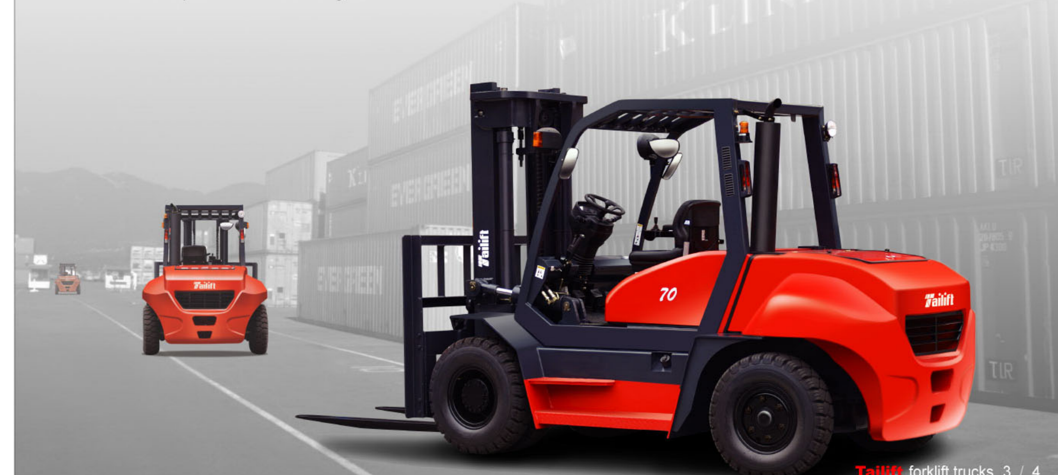
Wide visual head guard Driver gets a best visibility when operates lifting mast upward while watching the mast action.
