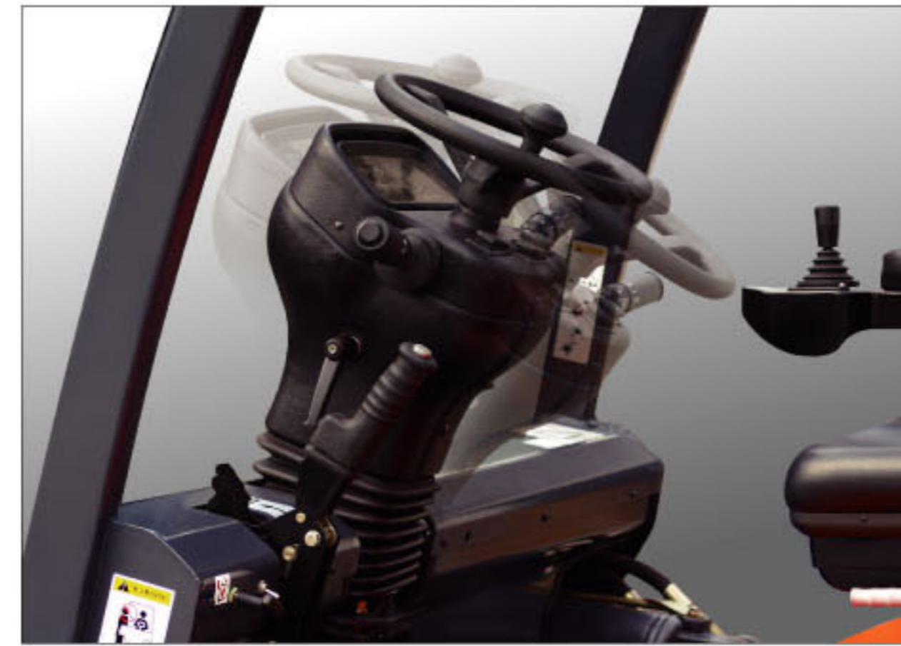
Tiltable Steering Column The steering column can be adjusted and to provide the preferred operating position.
