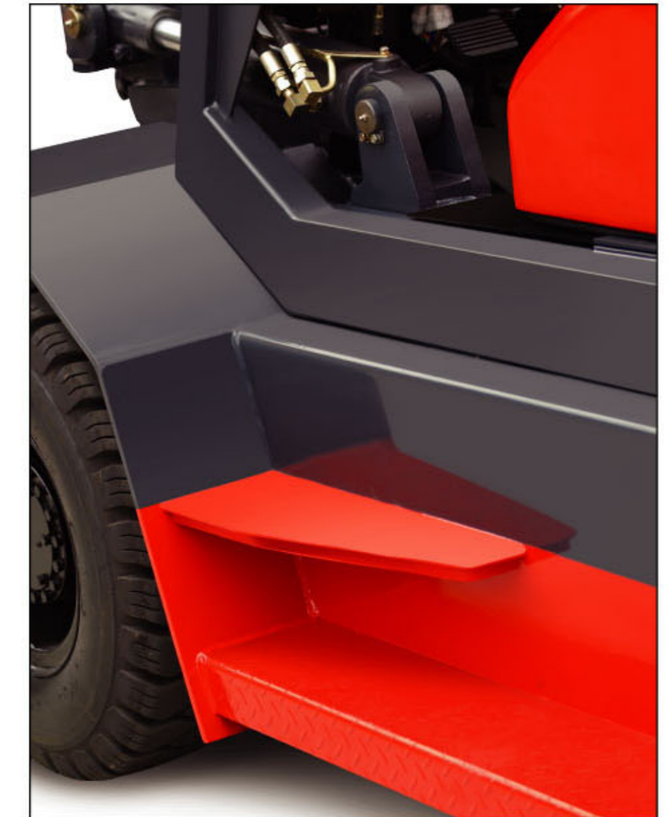
Easy Entry and Exit Low height from floor and secure non-slip steel step provides the operator easy step in and out of the forklift.
