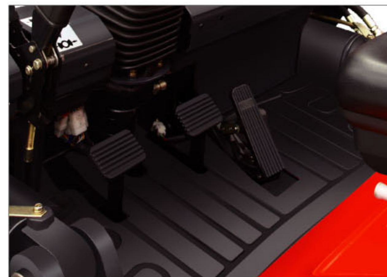
Electronic accelerator pedal Offering controllable engine speed and quick respond is to shorten timing of accelerating. Subvert normal cable pedal by electric pedal. Improve accelerator response speed.
